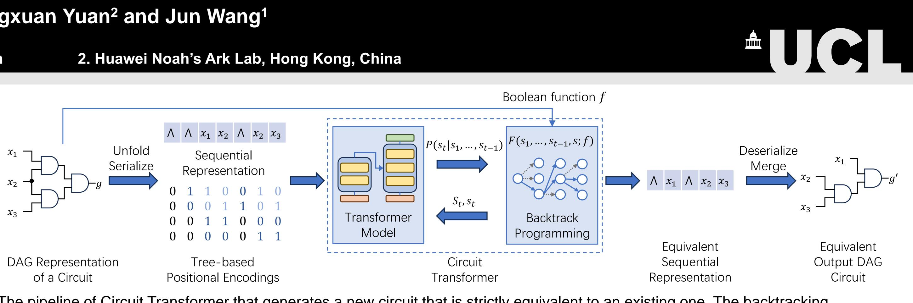
The pipeline of Circuit Transformer that generates a new circuit that is strictly equivalent to an existing one. The backtracking programming module acts as a masking layer at the end of the Transformer decoder.
